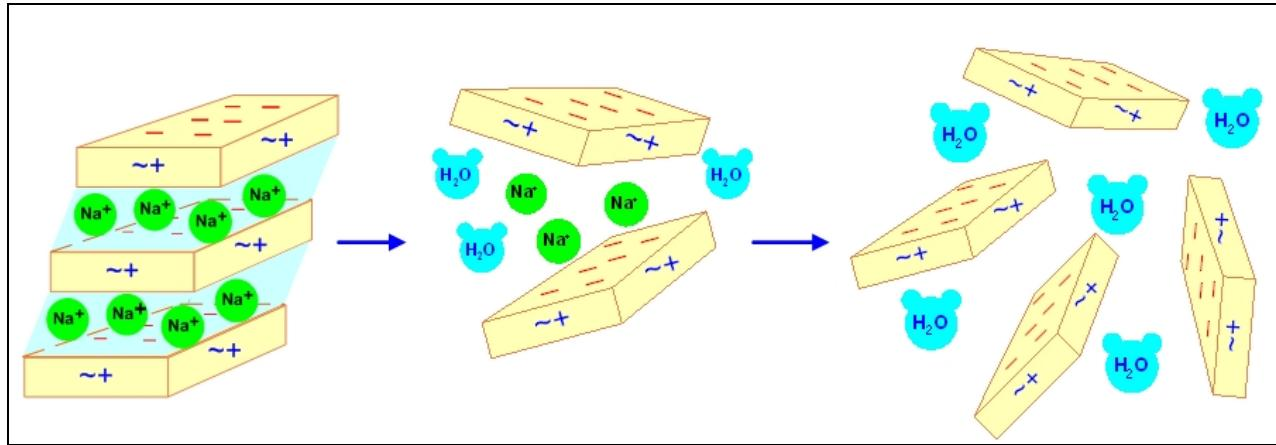
Hydraulic delamination of smectite clay
