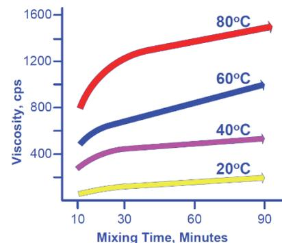
Any modification of mixer intensity (e.g., speed, propeller to vessel ratio) or water temperature will affect the degree of hydration and the hydration time. Whichever mixing conditions are used, it is very important that they be consistently controlled to achieve reproducible results in the laboratory, during scale-up and in production.
