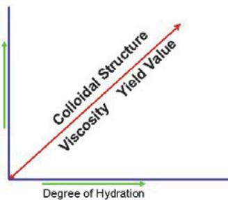
The degree of hydration is directly proportional to the amount of energy used to disperse the
