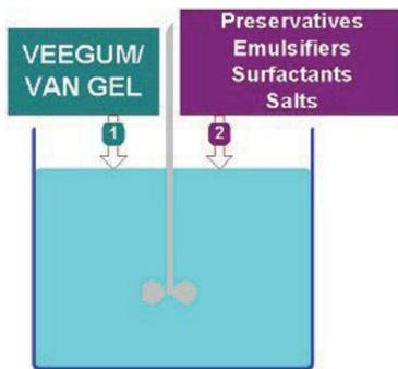
Dry clay particles are actually multiple layers of individual platelets separated by a layer of water. The extent to which these particles are delaminated into individual clay platelets is referred to as the degree of hydration. The greater the degree of hydration, the stronger the colloidal structure, and the greater the viscosity and yield value of the dispersion.
